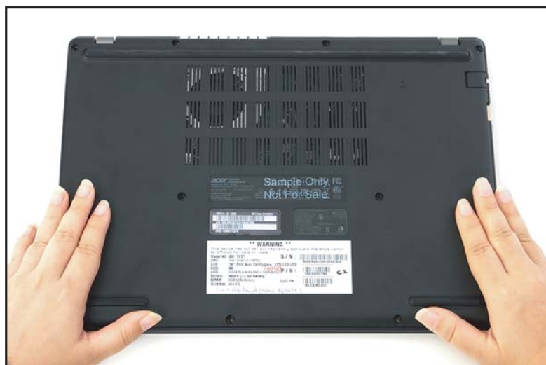
Figure 1-120. Replacing the Base Cover
