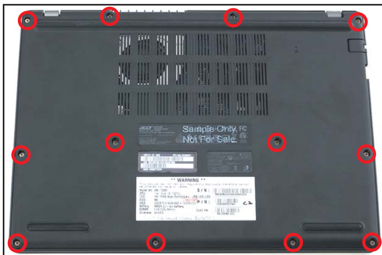
Figure 1-3. Base Cover Removal
