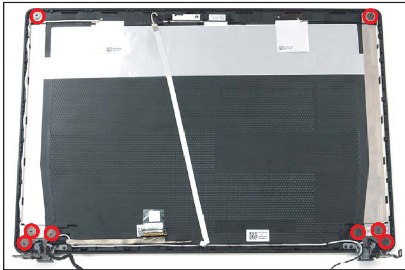
Figure 1-56. LCD Hinge Removal
