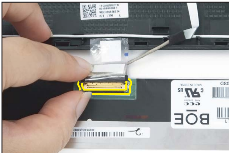
Figure 1-51. LCD Panel Removal
