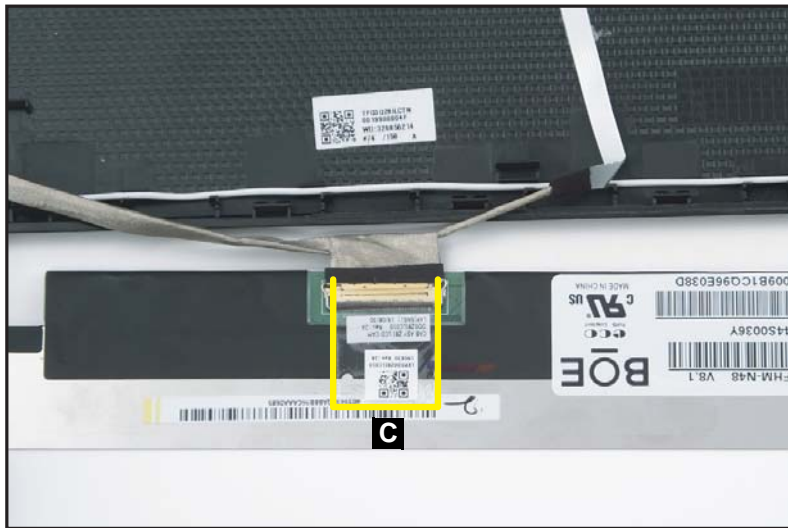
Figure 1-50. LCD Panel Removal
