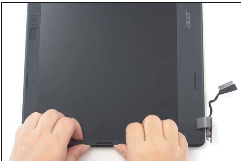
Figure 1-46. LCD Bezel Removal
