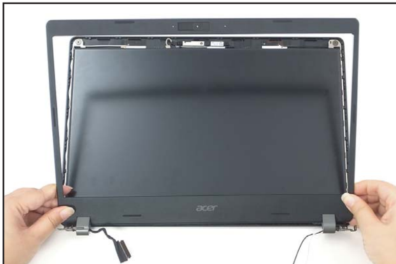
Figure 1-81. Replacing the LCD Bezel
