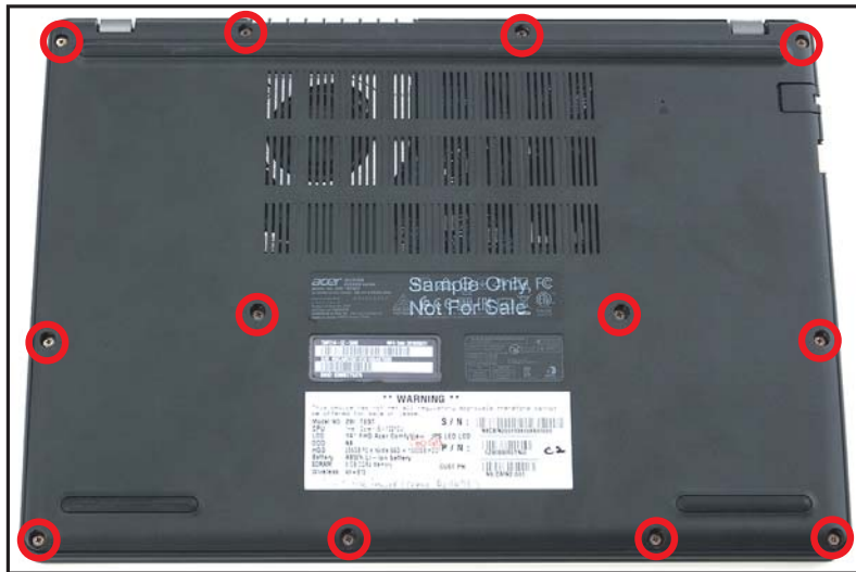
Figure 1-121. Replacing the Base Cover
