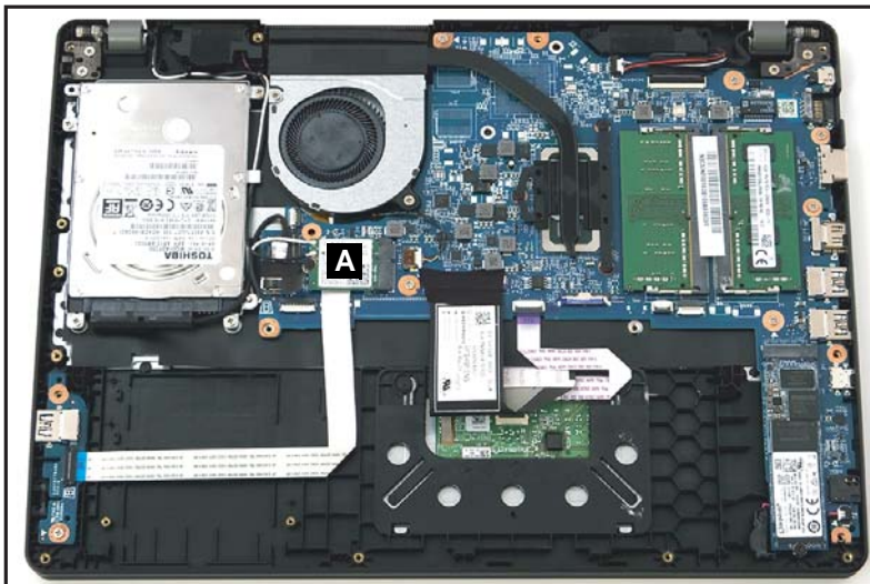
Figure 1-9. WLAN Module Location
