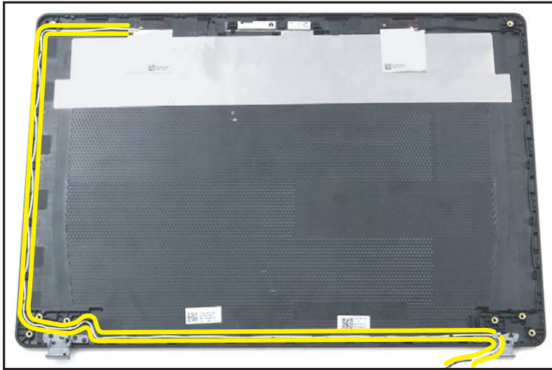
Figure 1-60. WLAN Antenna Removal
