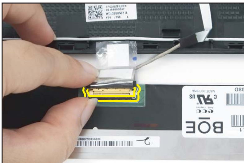
Figure 1-76. Replacing the LCD Panel
