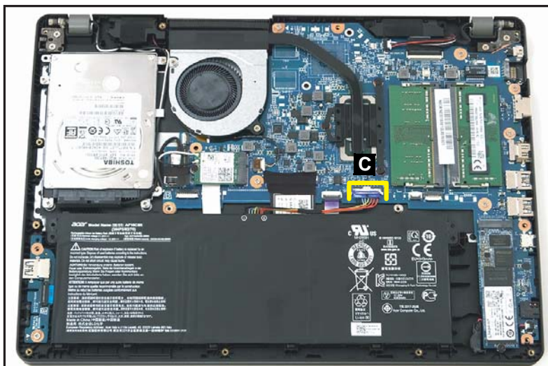
Figure 1-117. Replacing the Battery Pack
