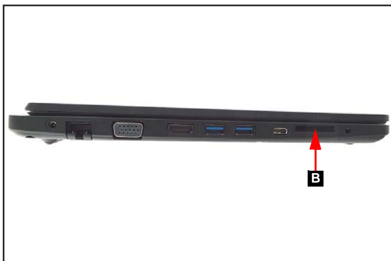
Figure 1-2. SD Card Removal
