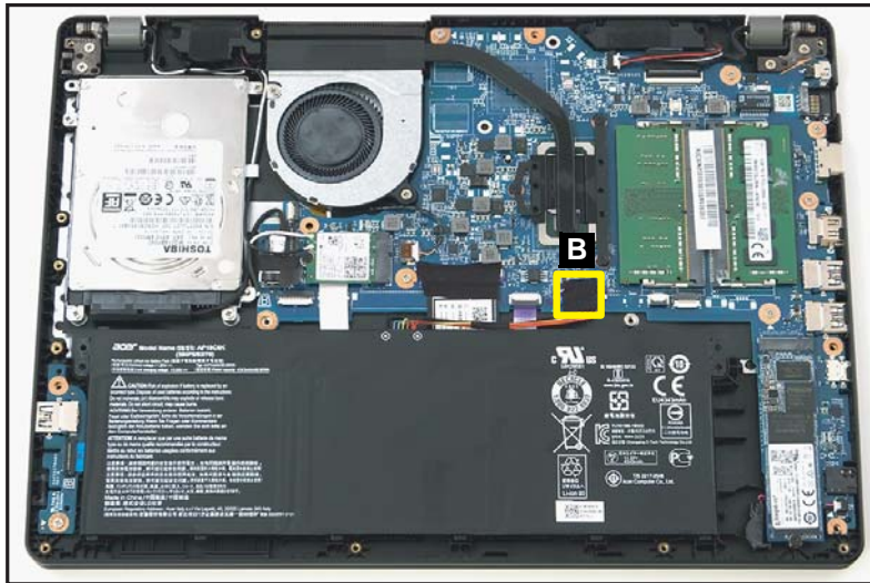
Figure 1-118. Replacing the Battery Pack
