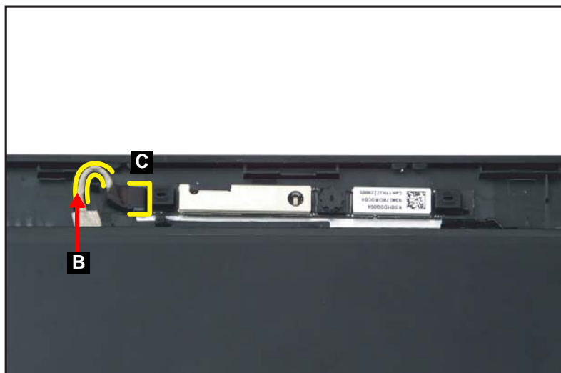
Figure 1-54. Camera Module Removal
