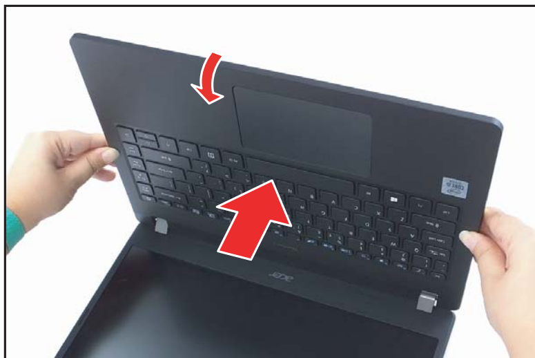
Figure 1-93. Replacing the LCD Module
