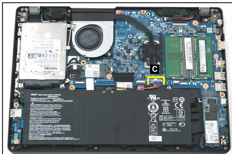
Figure 1-7. Battery Pack Removal
