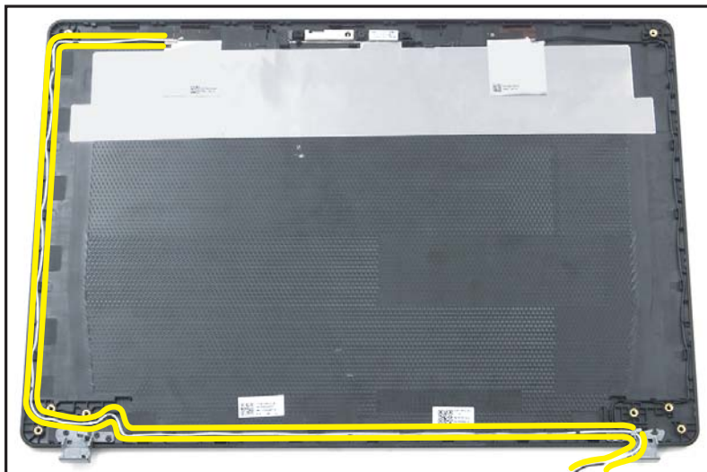
Figure 1-67. Replacing the WLAN Antenna
