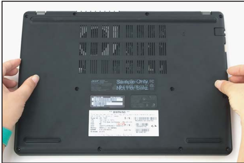
Figure 1-5. Base Cover Removal
