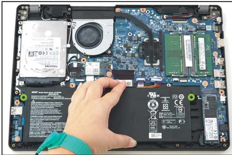
Figure 1-8. Battery Pack Removal
