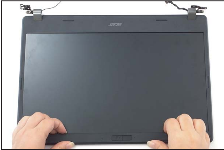
Figure 1-47. LCD Bezel Removal
