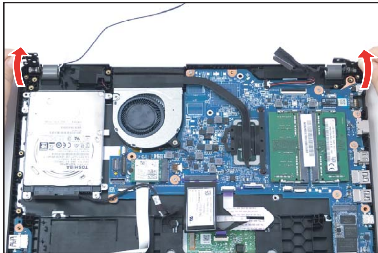
Figure 1-31. LCD Module Removal
