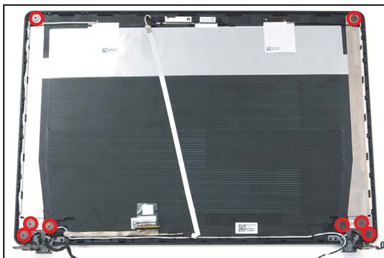
Figure 1-71. Replacing the LCD Hinges
