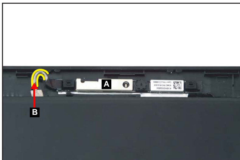
Figure 1-74. Replacing the Camera Module
