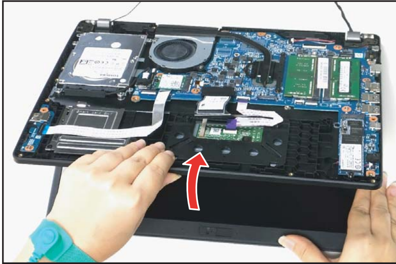
Figure 1-30. LCD Module Removal
