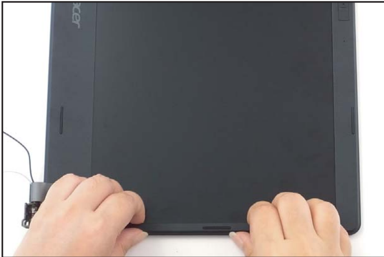
Figure 1-48. LCD Bezel Removal
