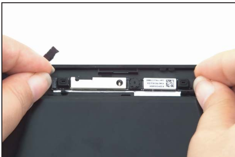
Figure 1-55. Camera Module Removal
