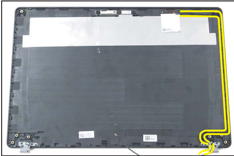
Figure 1-62. WLAN Antenna Removal
