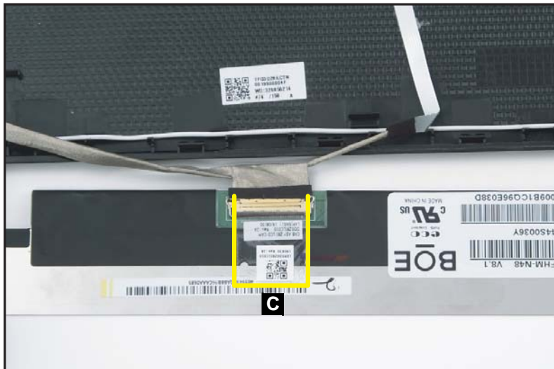
Figure 1-77. Replacing the LCD Panel
