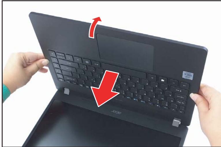
Figure 1-32. LCD Module Removal
