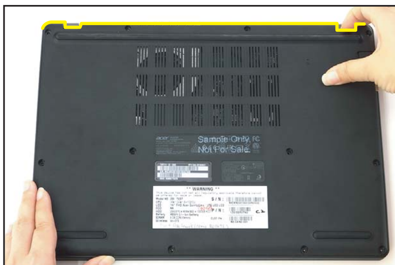
Figure 1-4. Base Cover Removal
