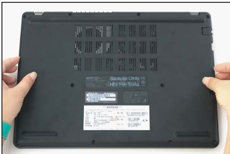
Figure 1-119. Replacing the Base Cover
